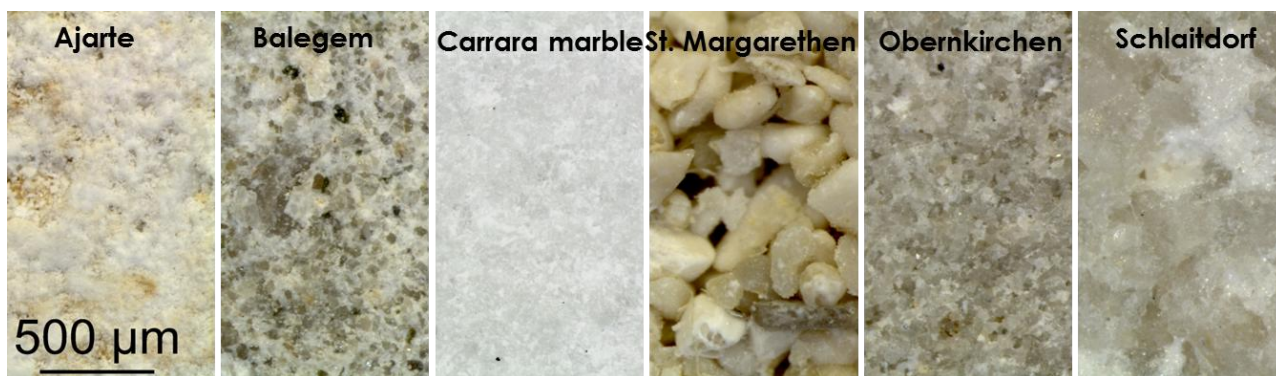
Fig. 1 – Microscopic images of Ajarte, Balegem, Carrara marble, St. Margarethen, Obernkirchen and Schlaitdorf specimens before the application of the protective treatments.
